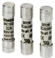
SITOR cylindrical fuse link, 22x58 mm, 80 A, aR, Un AC: 690 V, Un DC: 700 V, DC according to UL  $\,$
