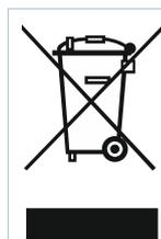
The device is considered an electronic device for disposal in accordance with the European Guidelines and may not be disposed of as domestic garbage.
